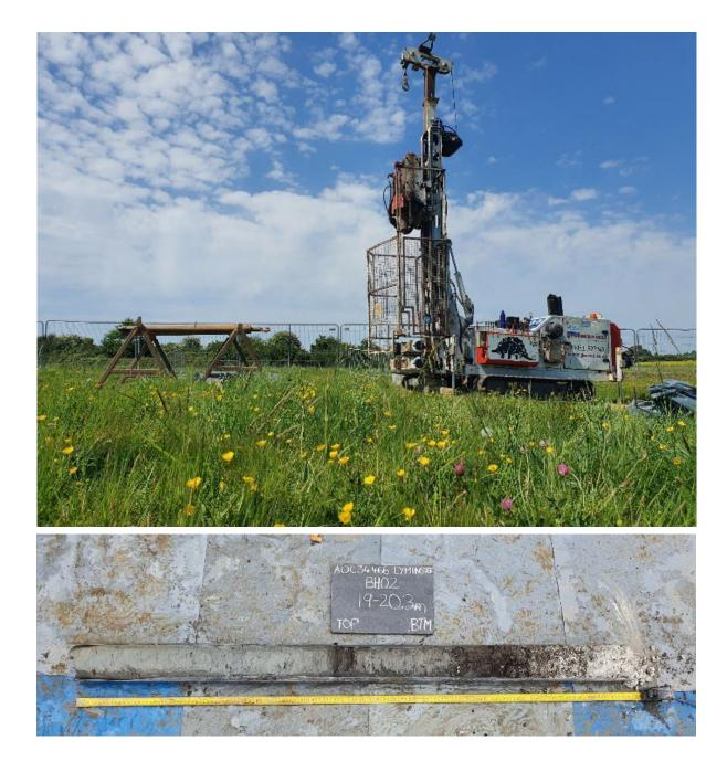
ABOVE: A machine drives a borehole through the 'Black Ditch' sediment. BELOW: A borehole sample showing different layers from the Black Ditch.
